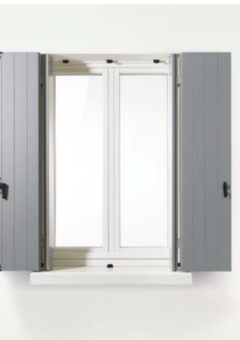
Serramento a due ante e scuro S20 dogato verticale in multistrato okoumè laccato RAL 7004, apertura alla padovana. Two-part shutter and S20 solid shutter with multi-layered vertical staves Okoume with RAL 7004 varnish, Padoan style opening.
